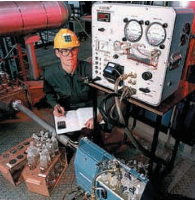
Figure 7. Flue gas sampling using EPA Method 29 for multimetals on the Powergen Combustion Test Facility (courtesy of Powergen)
