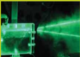
Probing the internal workings of a fuel cell: Laser Doppler anemometry mapping the flow of reactants inside a channel of an optically transparent fuel cell as performed in Dr Anthony Kucernak's research group, Imperial College London (Blewitt, Brett, Kucernak, Ladewig and Shrimpton). Image courtesy of Dr Anthony Kucernak, Imperial College London.
